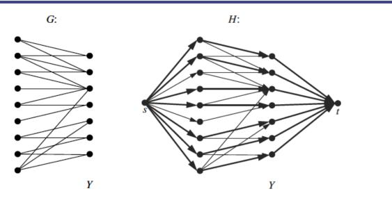
**Figure 16.11:** (a) A bipartite graph G. (b) Flow network H derived from G and a maximum flow in H; thick edges have unit flow and other edges have zero flow.
